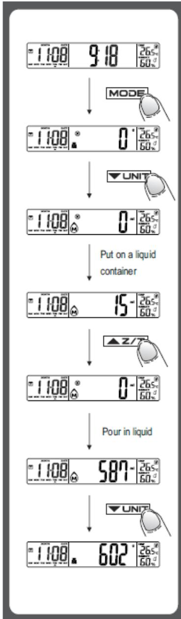
This scale can convert the weight of milk and water automatically into volumes measurements (ml or Fl. Oz).
